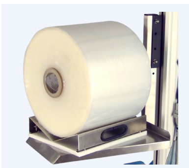
Platform with V-block, combined with the rotating disk, rotates the V-block so that the roller can be positioned correctly.
