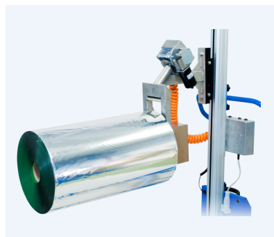
Pneumatic expander, lifts at the center, it's expandable 360°.
