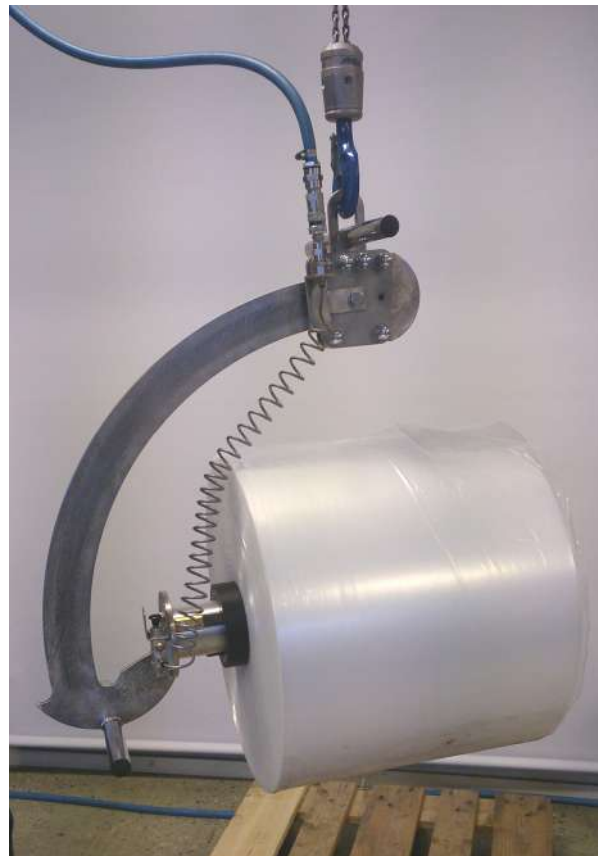
Transport to unloading point. Make sure the roll is secured when dropped off.
