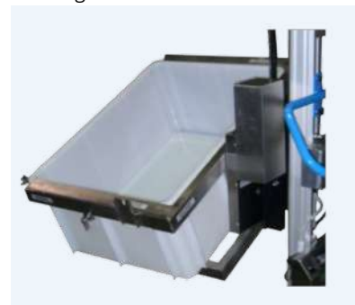
Customized clamping tool that can be rotated 360°.
