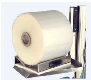
Platform with V-block, combined with the rotating disk, rotates the V-block so that the roller can be positioned correctly.
